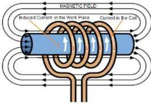
Fig. 1: The principle of conventional inductive heating
