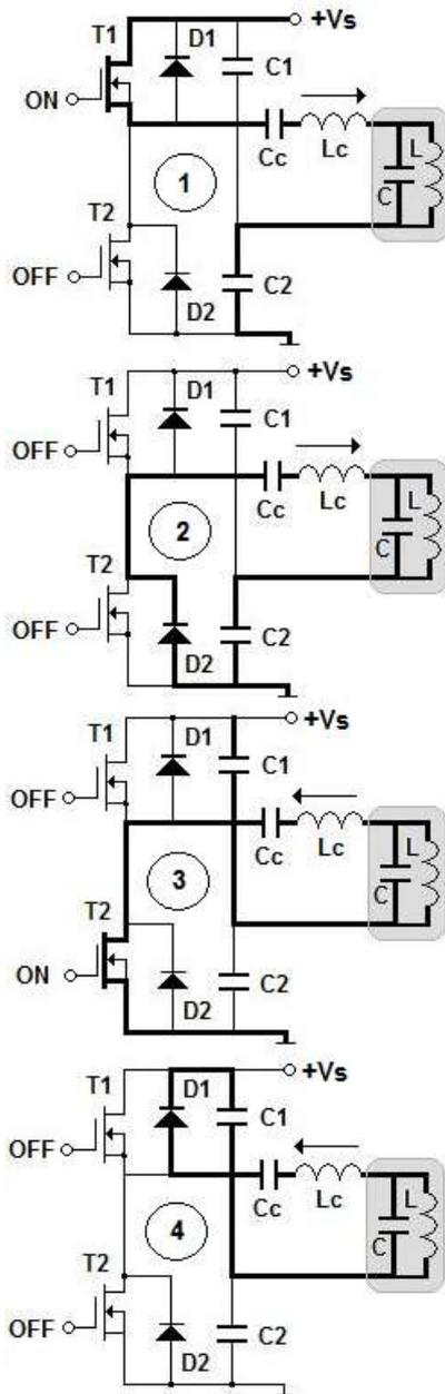
Fig. 3: The command of half bridge sinusoidal inverter
